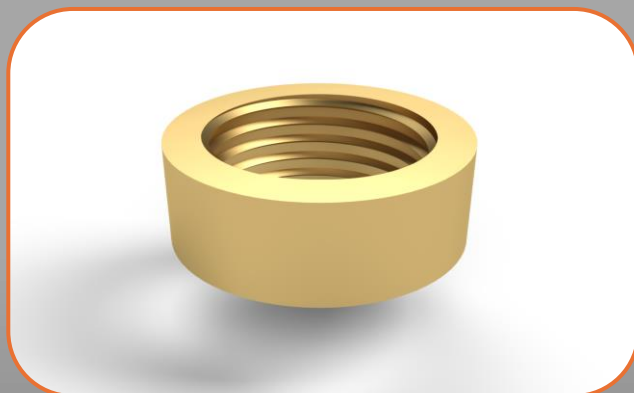
Offset surfaces from derived body ensure compatibility with standard Jetboil propane canisters.
