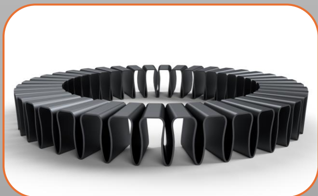
Surface modeling used to capture complex curvature of flux ring.
